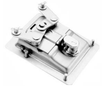
'Blind-mounting' models have four studs (M6 x 15 mm) welded on inside flanges
